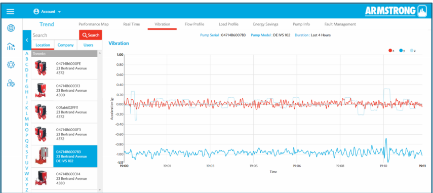
Real Time Vibration Tracking
